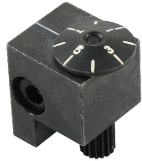
**Note: You simply cannot use the threading dial when cutting metric threads. Leave the lead screw engaged all the time. When you are done with a pass, note the position of the cross slide dial. Back the cross slide out about two turns. Then run the lathe in reverse until you are back at the starting point.**
